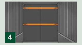
Two deck bars are dropped in front of the panels. The empty space can be filled with air bags.
