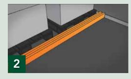
A frame is placed on the trailer floor against the freight. This frame consists of two 2 x 12s and one 1 x 8.
