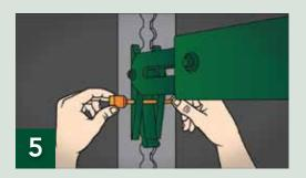
A lock is placed in the drilled hole of one of the deck bars.
